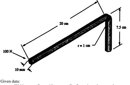
Width across flats = 10 mmConfiguration = hexagonalLength of shank = 7.5 cmLength of handle = 20 cmBend radius = 1 cmModulus of elasticity =  $2.07 \times 10^5$  MPaApplied tangential force = 100 N
