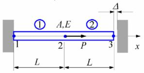
Problem: Determine the support reaction forces at the two ends of the bar shown above, given the following,
