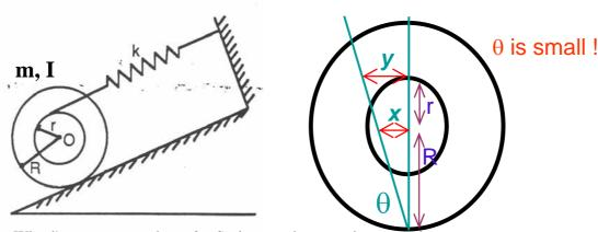
Wheel's centre moves by x & Spring attachment point moves by  $y \otimes Spring$
